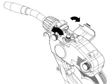
• Rotate the tension arms away from the main drive roller.
