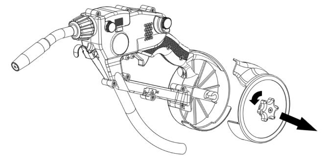
Step 2: Move the spool brake to the locked position:
