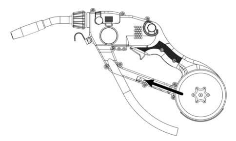
Rotate the spool brake lock (9) downward into the locking notch:
