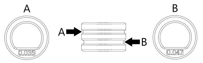
If using 0.030" or 0.035" welding wire, the 0.035" groove should be used. This groove has been designed to accommodate both wire diameters.
